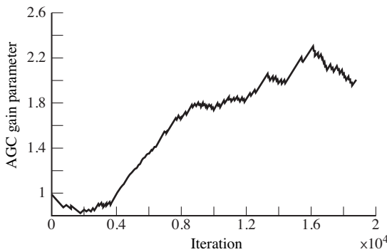
Figure 9.12 Trajectory of the AGC gain parameter as it moves to compensate for the fade.
