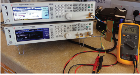
Figure 3. Measurement setup with two signal generators.
